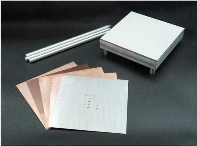
The resolution plate has four columns of five holes each with hole diameters of the following sizes:
