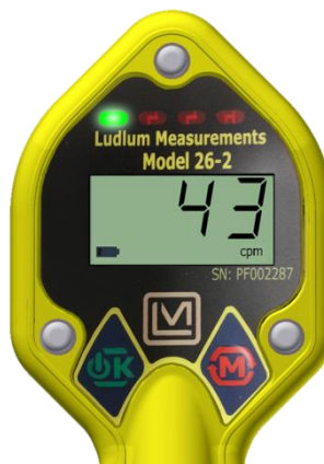
Figure 1: RATE mode display showing typical background radiation rate and the low-battery icon. Green LED will be flashing.
