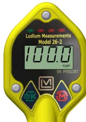
Figure 2: Detector Over Range (shown for cpm); will also flash.
