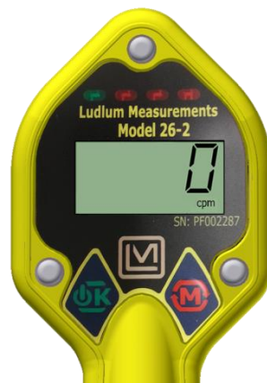
Figure 2: Detector Failure display (shown for cpm); will also flash.
