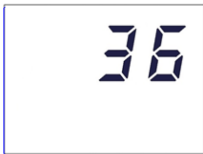
Figure 5.2: Displaying Datalog Location ID Table Index of 36
