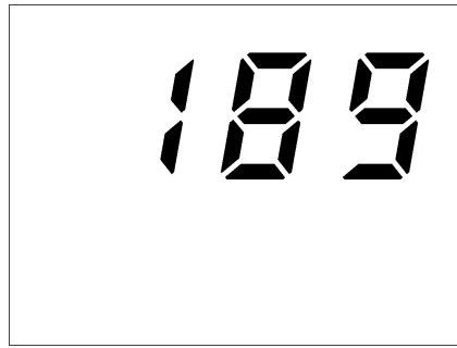
Figure 2.5: Startup Display Showing 189 Stored Data Records
