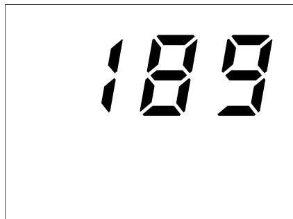
Figure 2.4: Startup Display Showing 189 Stored Data Records
