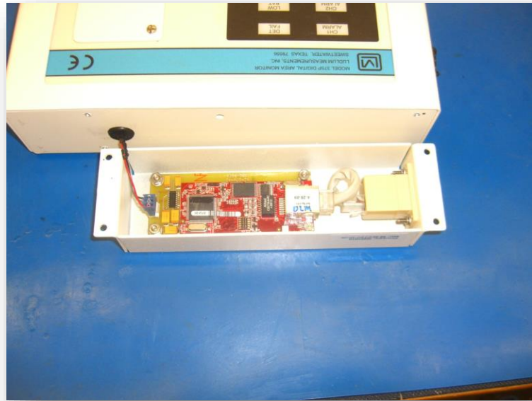
Figure 45 – External Rabbit Ethernet Board Removal
