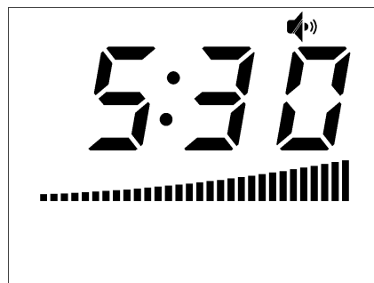
Figure 2.16: COUNT Mode Displaying COUNT Timer of 5 Minutes, 30 Seconds
