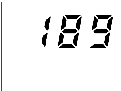
Figure 2.5: Startup Display Showing 189 Stored Data Records
