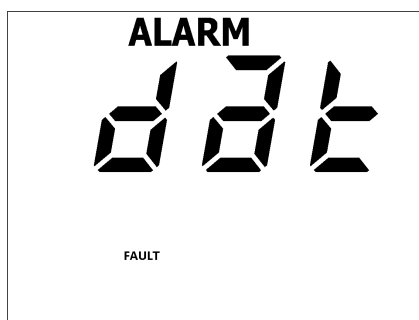
Figure 2.6: Instrument Date Reset (Audio Alarm)
