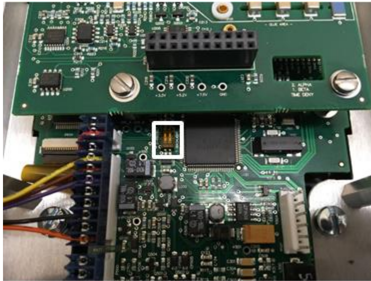
Figure 4.1: Backlight/Setup Protect Dipswitch
