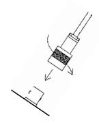
The detector operating voltage (HV) is supplied to the detector via the detector input connector. A mild electric shock may occur if you make contact with the center pin of the input connector. Switch the Model 12 range selector switch to the OFF position before connecting or disconnecting the cable or detector.
