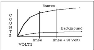
**Proportional Detectors**: Set the DIS control for 2-millivolt discrimination (near maximum clockwise). Expose the detector to a check source. Adjust the HV until the low-energy source is detected. Refine the HV adjustment for an optimum source count with a minimum acceptable background count.
