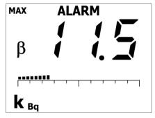
Figure 2.9: MAX Mode Display With ALARM Indication
