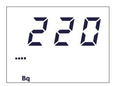
Figure 2.2: Firmware Version Display
