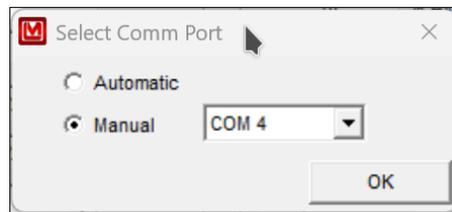
When the software is started, a dialogue is displayed allowing the user to manually select the Comm port or to have the software select it automatically. The software will only search Comm ports 1-16. After the Model 3030 is found, the parameters are downloaded from the instrument and the main screen is displayed. The main screen consists of a tabbed interface separating the various functions and includes General Settings, QC Check, HV Plateau, MDA Calculation, and Data Logging.
