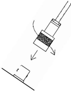
Connect one end of a counter cable to the counter by firmly pushing the connectors together while twisting clockwise a quarter of a turn. Repeat the process in the same manner with the other end of the cable and the instrument.
