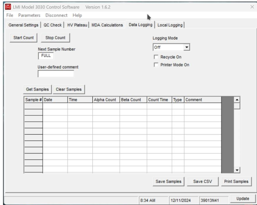
The Model 3030 can store 600 samples in its data logging memory. The following fields are stored with each sample: time, date, alpha reading, beta reading, count time, count mode, and user-defined comment.
