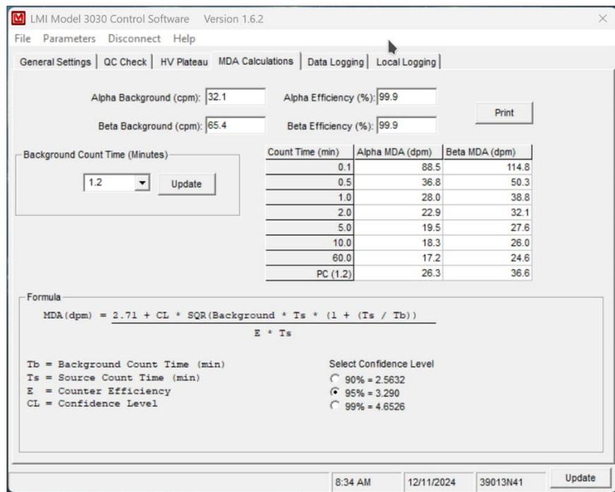
This screen shows the calculated MDA values for all count times based on the current background and efficiency values. The confidence level may be set at 90%, 95%, or 99%. This screen is only available when the instrument is in DPM mode. The values are preset according to the current instrument settings but may be changed here. The data may also be printed to a printer.
