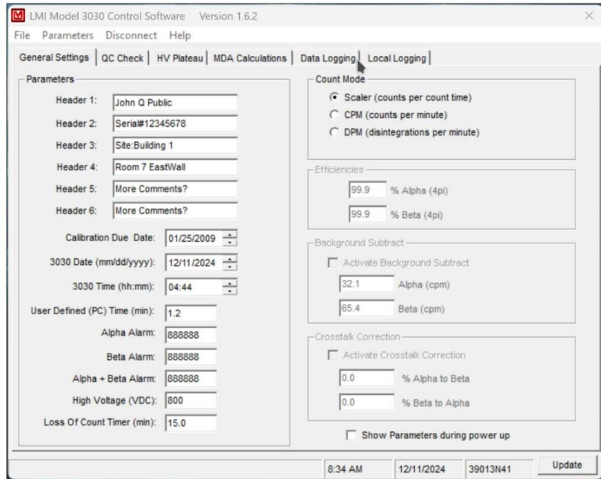
The following parameters require a password: Calibration Date, Date, Time, High Voltage, Background Subtract On/Off, Alpha Background Subtract, Beta Background Subtract, Alpha Efficiency, Beta Efficiency, Crosstalk On/Off, Alpha Crosstalk, and Beta Crosstalk. Running an HV Plateau is also password protected.
